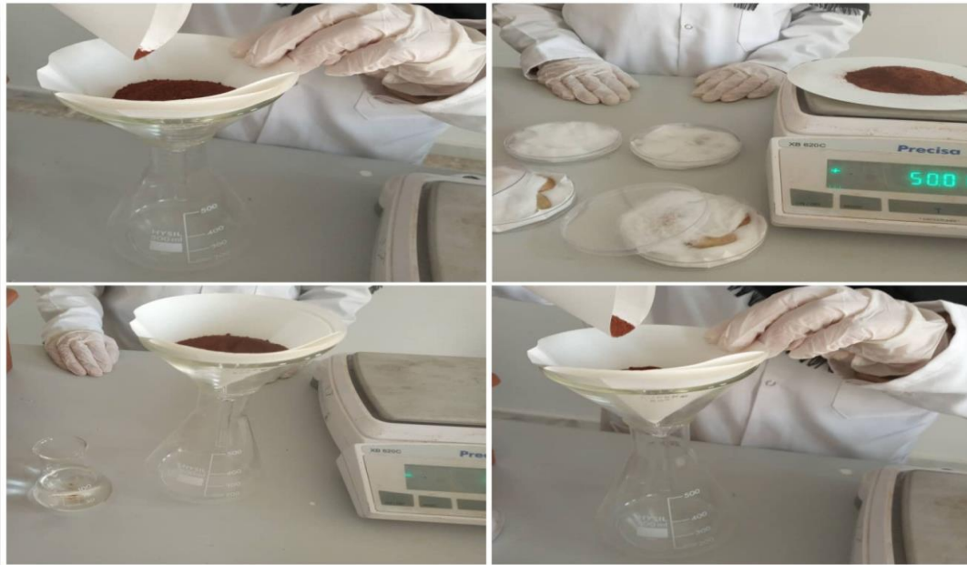
Figure (1) adjusting the water content and calculating the field capacity of the soil
