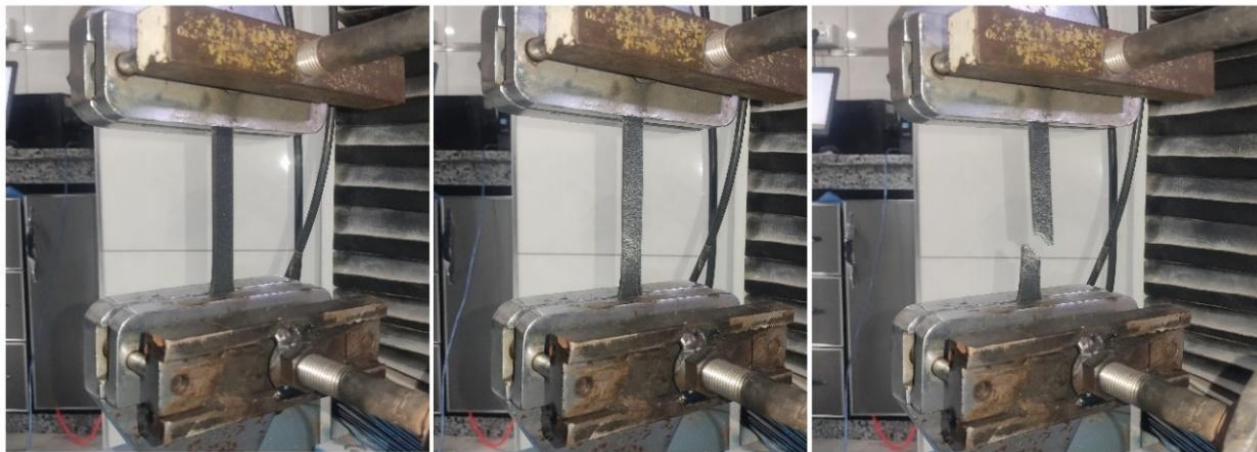
Fig. 14 The polymer sample being installed on the jaws of the tensile testing machine.
